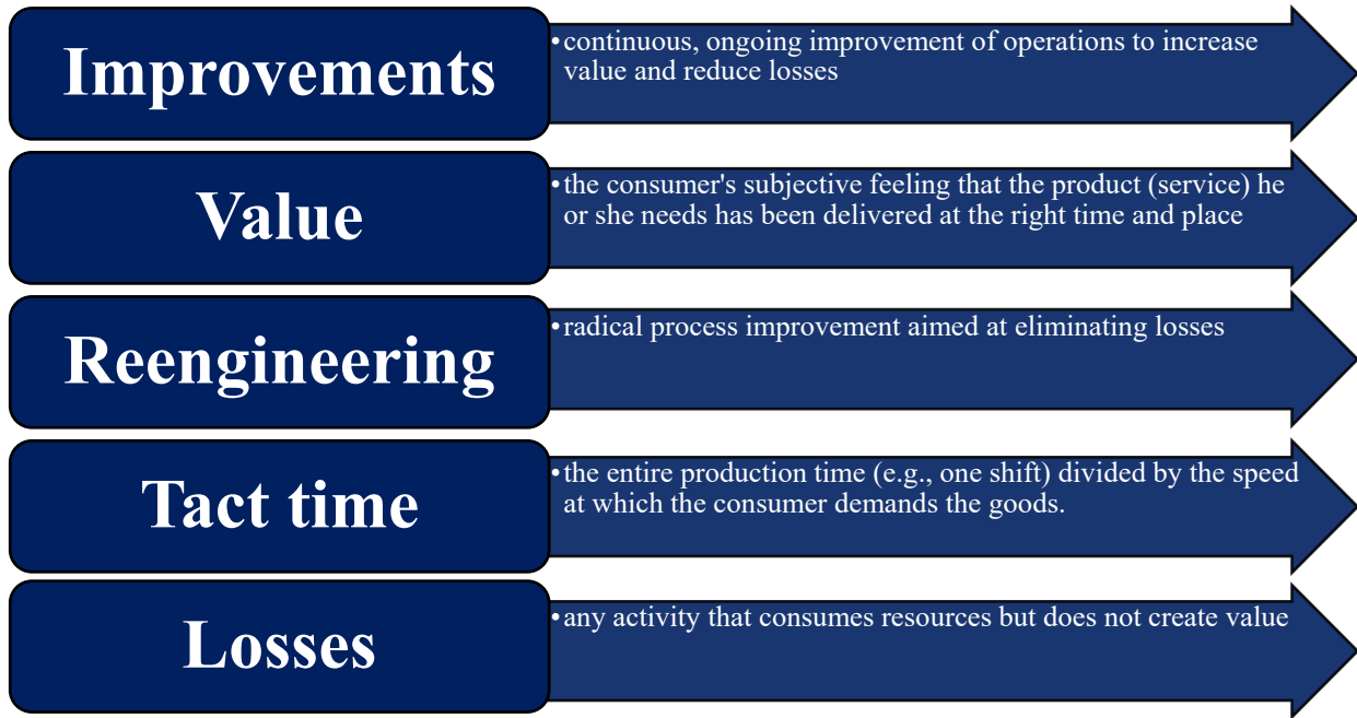
Fig. 3. Key concepts of “Lean technologies” Source: developed by the authors on the basis of [8–9]
