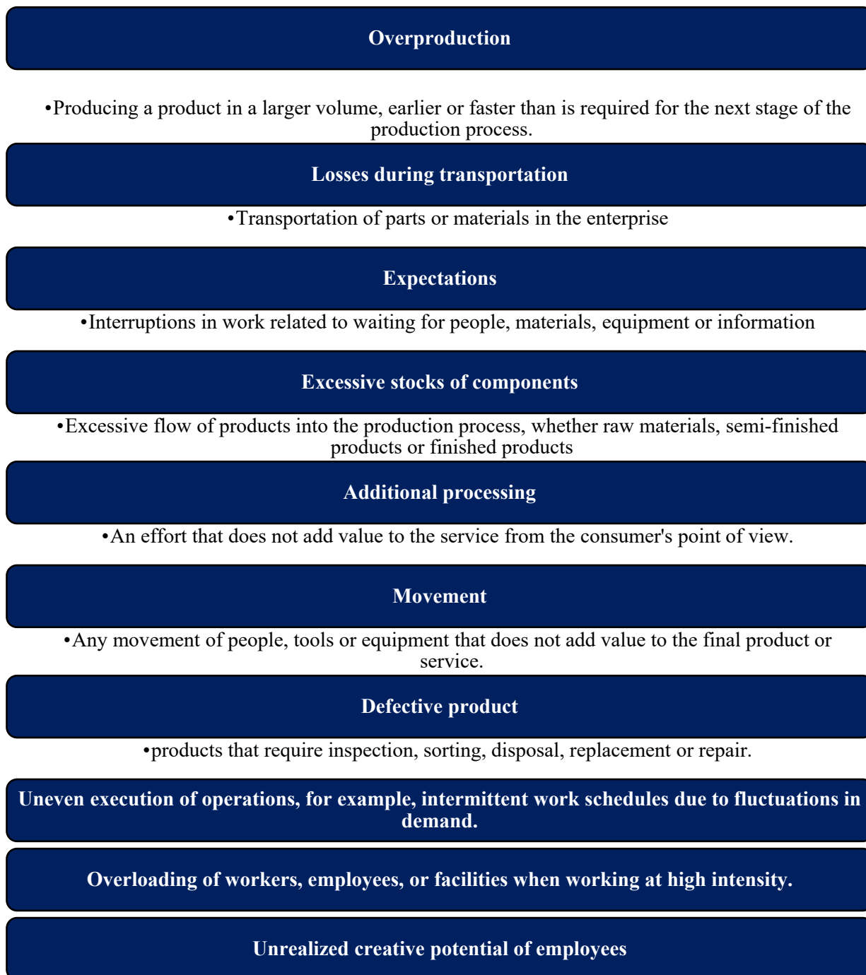
Fig. 2. Losses that are eliminated when implementing the Lean production concept Source: developed by the authors on the basis of [6–7]
