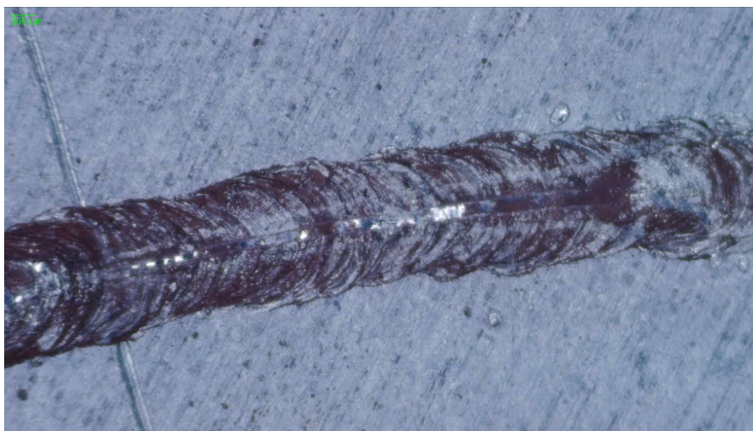
Fig. 5. The appearance of the closure area of the annular seam during laser welding
